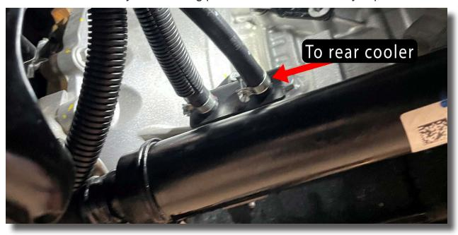
1.29. Secure using cable ties provided. Remove all clamps and replace the plastic panel that was removed from the wheel arch and refit bash plate.
