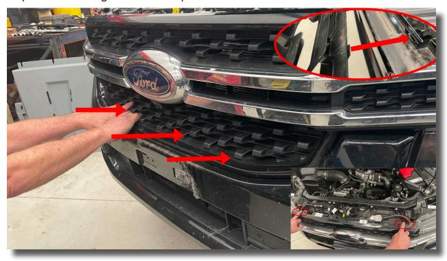
1.31. Reconnect the 2 plugs above the grill for the front facing camera and washer. Don't forget to top up the washer bottle!
