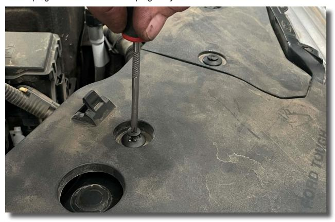
Using a T30 Torx bit, remove the screw holding the air inlet manifold to allow you 1.4. to easily remove and reinstall the radiator cover.
